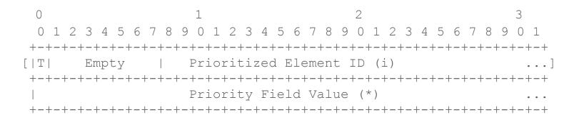
**Initially** sent on the request stream before headers Reprioritization on the control stream
