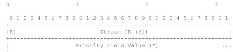
**Only** sent on the control stream, because of HTTP/2 extension constraints MUST be sent immediately preceding corresponding headers
